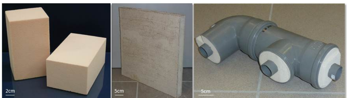
Examples of porous alumina (density 0.36\text{g/cm}^3 , left), porous gypsum panel (density 0.25\text{g/cm}^3 , middle) and a complex-shaped tube insulator also made from porous gypsum (right).
